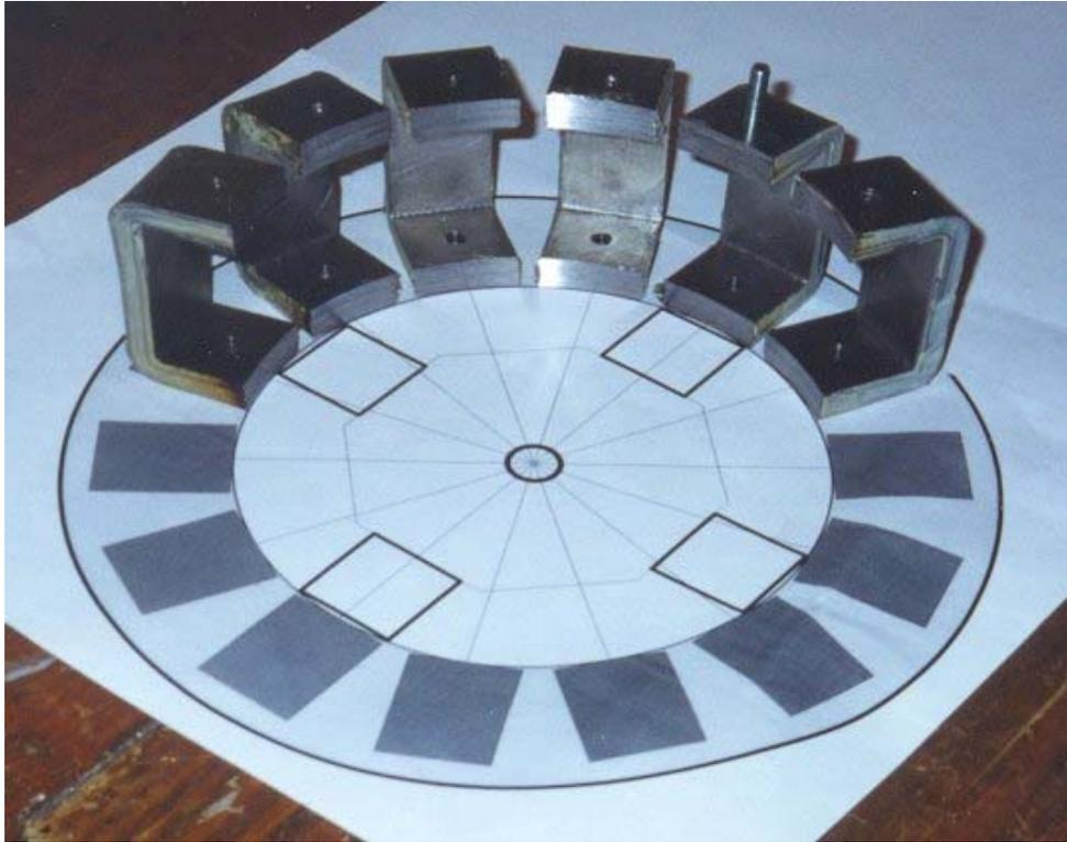
Partial (unwound) stator core assembly
