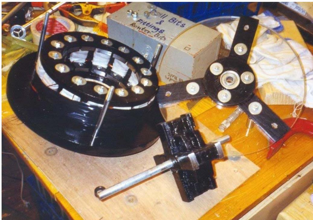
Stator assembly, rotor assembly, and motor top plate
